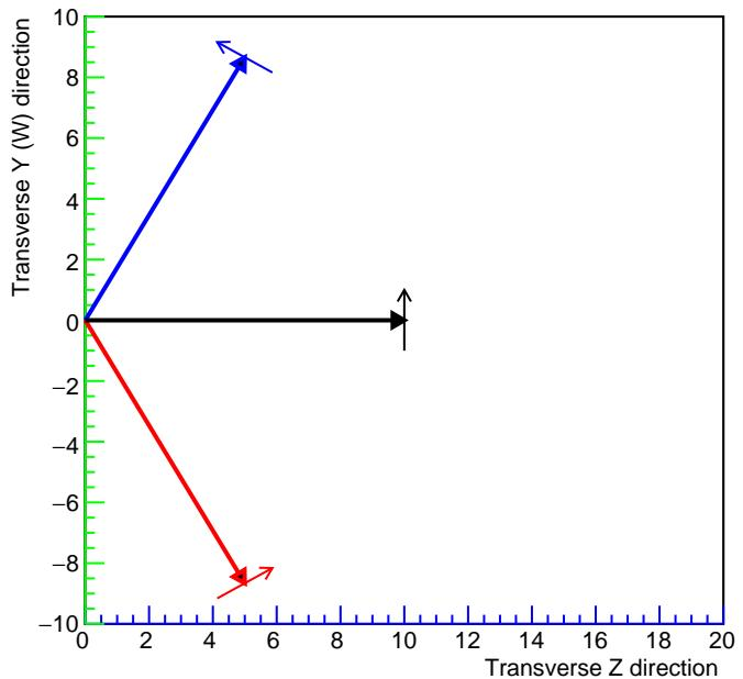
Pitch (thick) and wire (thin) red=U, blue=V, +X (-drift) direction into page
