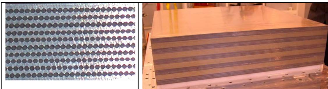
Fig : detail of the lead/scintillating fiber sandwich (left) and (right) pancake before assembly in the mechanical support structure.
