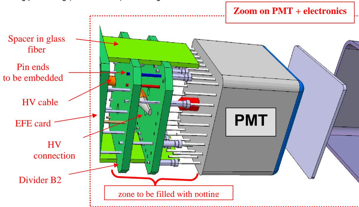
All the HV pins or connections are embedded in DC 93-500 potting. The process as described in the Annexe 3, is an injection of pre-outgassed DC93-500 through a transparent PMT box (visual inspection). Quality check: 1. Visual Inspection during injection (air bubbles), 2. Thermal Vacuum tests for each PMT Tube. All HV cables are protected both with potting and shielding in Teflon.
