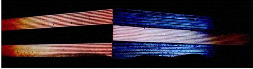
**Figure 5.11-1 Three Superlayers Showing Alternating Layers Of Lead Foil And Scintillating Fibers And Alternating Superlayer Orientation**
