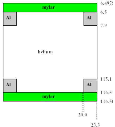
Figure 2: Geometry for simulation of helium filled mylar bag with Al rings. Distances in centimeters.
